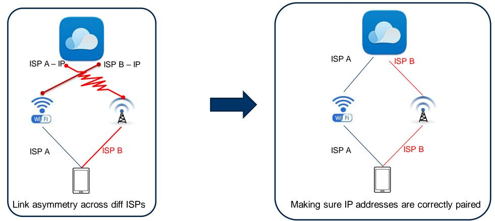
Problem: subflows established between IP addresses of different ISPs will result into longer delay and path discrepancy.
